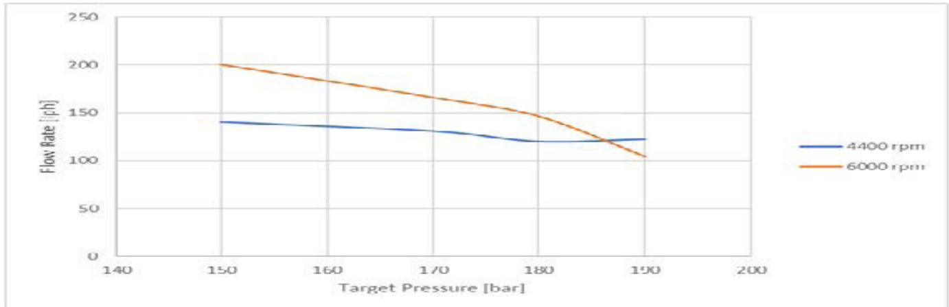
**Fig 3- Target Pressure vs Flow Rate**
