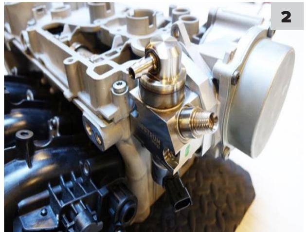
3. Obtain the two stainless steel M6 x 45mm long Allen bolts from the kit and align the pump main body bolt holes to the threaded holes on the flange. Insert the bolts and hand start them.
