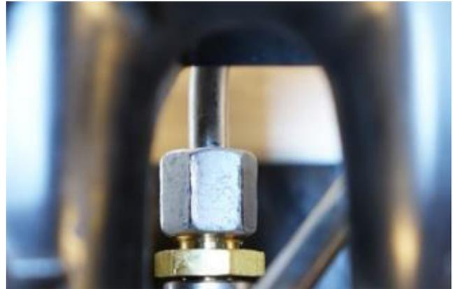
**NOTE:** You may need to remove the airbox and wiring harness clip to gain access to the fitting from underneath the intake manifold. This is the best way to get an open-end wrench to the fitting. See your OEM maintenance manual.
