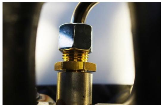
11. Attempt to move or shake the high-pressure hard line at both ends near the fittings. They should not move inside the compression nut. If they do move, remove the tube and go back to Step 8.
