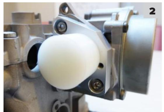
**TIP: Rotate the installation tool while seating the two fasteners. This will assist in preventing the installation tool from becoming trapped and difficult to remove.**
