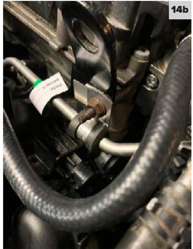
14. After tube is installed) Align the rubber-lined P-clamp with the “Z” bracket and fix them together with the provided M6 bolt & nut. **Torque the bolt to 9 ft-lb.** (See fig. 14a and 14b)
