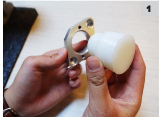
2. Insert the installation tool into the pump bore on the cylinder head (vacuum pump housing). Be sure to gently slide into the bore. The installation tool will align the flange and the O-ring into proper orientation and concentric alignment with the pump bore on the cylinder head. This prevents O-ring damage, pump damage, and pump installation problems. Push into the bore until the flange and O-ring are seated against the pump mounting face on the cylinder head. **See fig. A**
