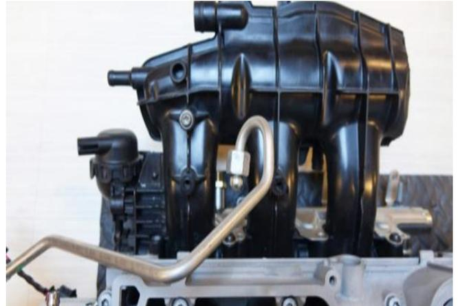
9. Next, ensure the spherical fitting is seated and aligned on the FUEL PUMP side. While holding the FUEL PUMP fitting in place, align the other end of the hard line spherical fitting to the FUEL RAIL female cone. **IT IS IMPORTANT TO ENSURE THE FUEL PUMP FITTING IS SEATED FIRST, THEN SEAT THE FUEL RAIL SIDE.**
